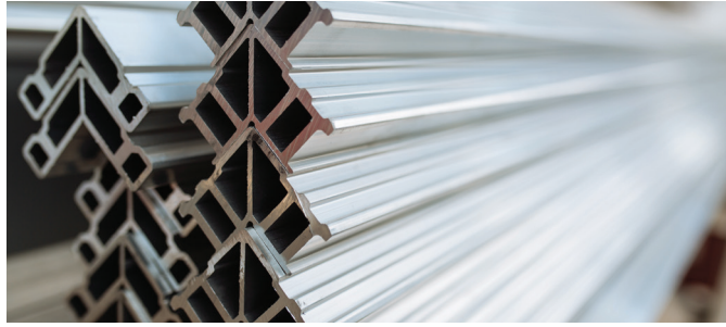
Aluminum extrusions are coated and cut into sections to build products such as window frames. This process also leaves edges of metal uncoated and unprotected from moisture, salt and other hazards that cause corrosion.
