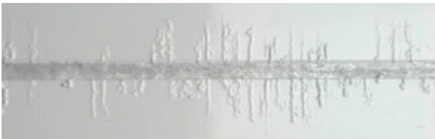
Example of filiform corrosion creepage away from a horizontal exposed scribe
