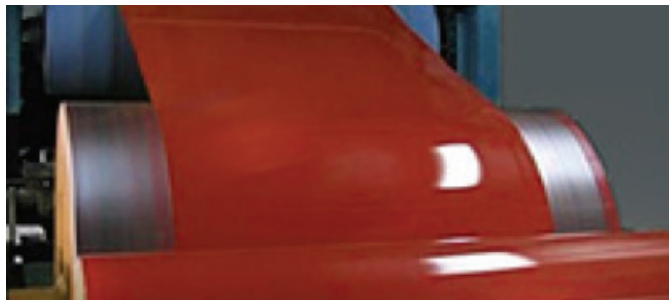
Coil coatings are applied to the surface of metal building products by roll-coating, which leaves edges unpainted and vulnerable to corrosion when the product is transported, stored outdoors or installed on a building.
