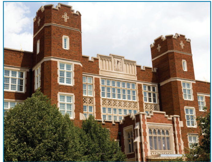
Nearly 2,000 windows on Washington, D.C.'s historic Eastern High School were restored or replaced with units featuring Duranar coatings and Solarban 60 glass.
